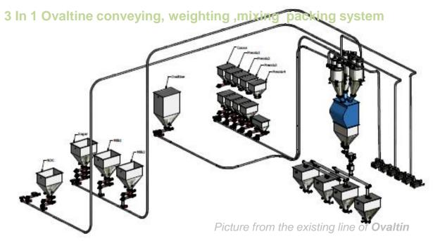
Full Bulk material handling system for food grade powder and bulk processing line / Storage / Loading / Unloading / Weighting / Mixing / Sizes classifying Connecting all together by pneumatic conveying system and control.
